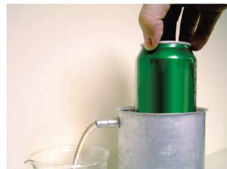
Figure 2. Collecting the displaced water as the soda can is slowly lowered into the overflow container.
