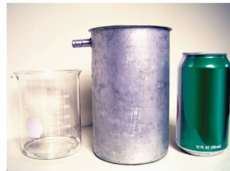
Figure 1. Materials for measuring the volume of displaced water (glass beaker, aluminum overflow container, and unopened soda can).
