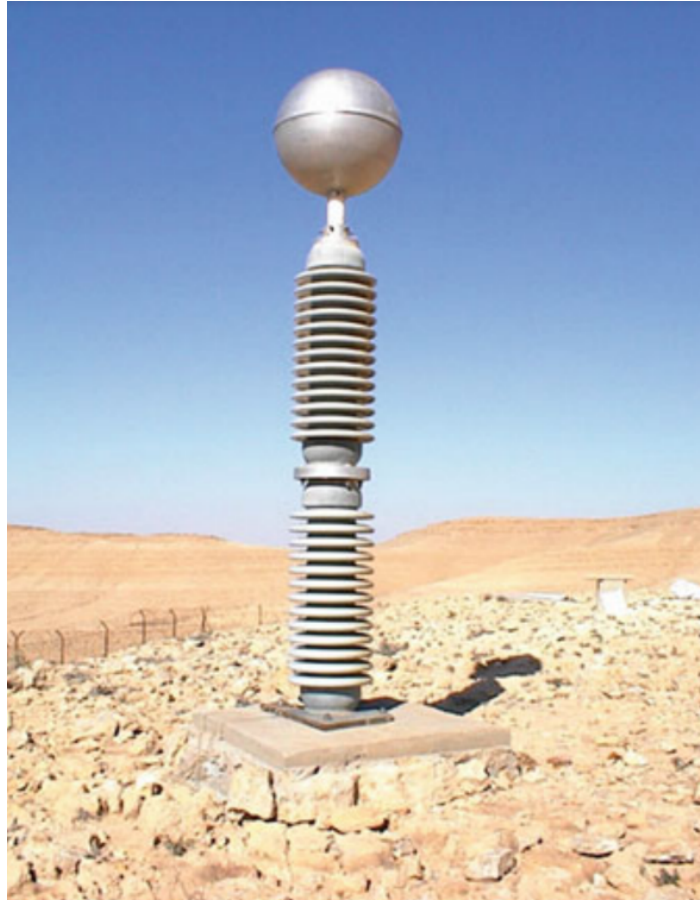
Figure 1.4: Ball antenna for electric field measurements in the ELF range in Mitspe Ramon Observatory (Israel), extracted from Nickolaenko and Hayakawa (2014) [4].
