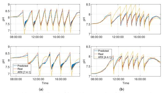
**Figure 4.** Validation results for each of the models using two days of the test set. (**a**) Freshwater model validation results, (**b**) Wastewater model validation results.
