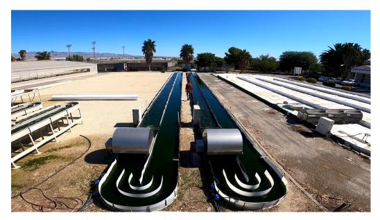
Figure 1. Raceway photobiorreactors modeled in this work.
