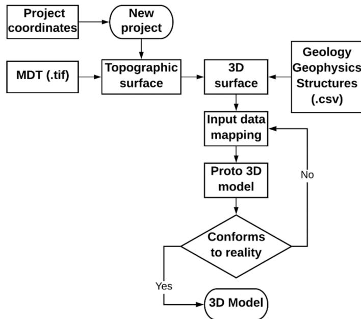
Figure 5. GeoModeller software process creation model.
