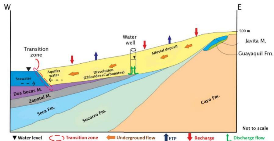
Figure 7. Alluvial conceptual model. Modified from the study [44].
