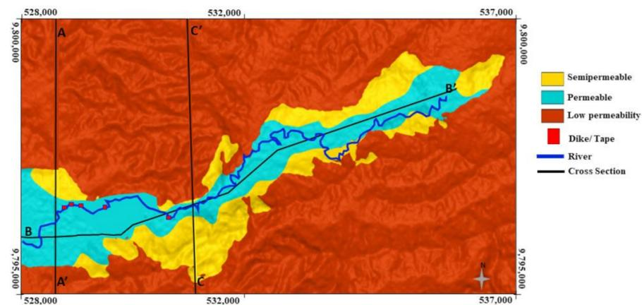
Figure 8. Plan view of the hydrogeological units modeled.
