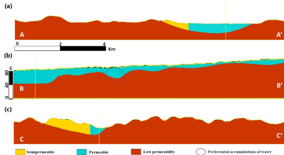
**Figure 9.** (a) A–A’ cross-section of the lower part, in the broadest area of the alluvial. (b) B–B’ cross-section along the permeable zone shows the water accumulations’ geometry, highlighting the preferential accumulations. (c) C–C’ cross-section of the geometry of the preferential accumulations of water.
