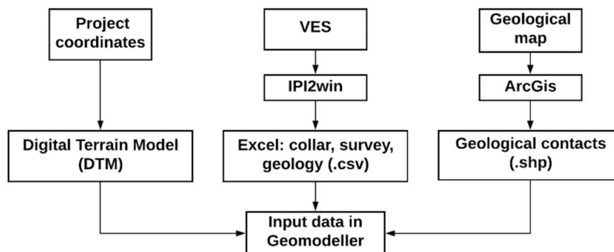
Figure 4. Input data schema in the GeoModeller software.
