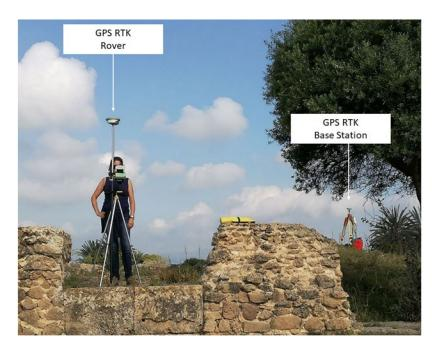
**Figure 19.** Measurement of control points with GPS RTK for photogrammetric flight in the city of Utica (Tunisia).
