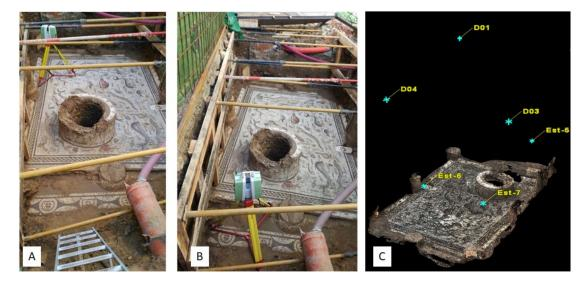
**Figure 20.** Roman mosaic in Cantillana, Seville (Spain). (**A**,**B**) Measurement of points by laser scan at different positions. (**C**) Result as cloud of points.
