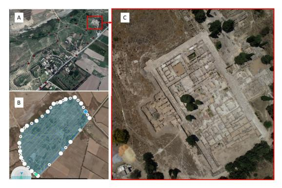
**Figure 15.** UAV photogrammetric flight of Utica (Tunisia). (**A**) Ground control points. (**B**) Photogrammetric flight paths. (**C**) Example of aerial photography on the restored Roman insula.
