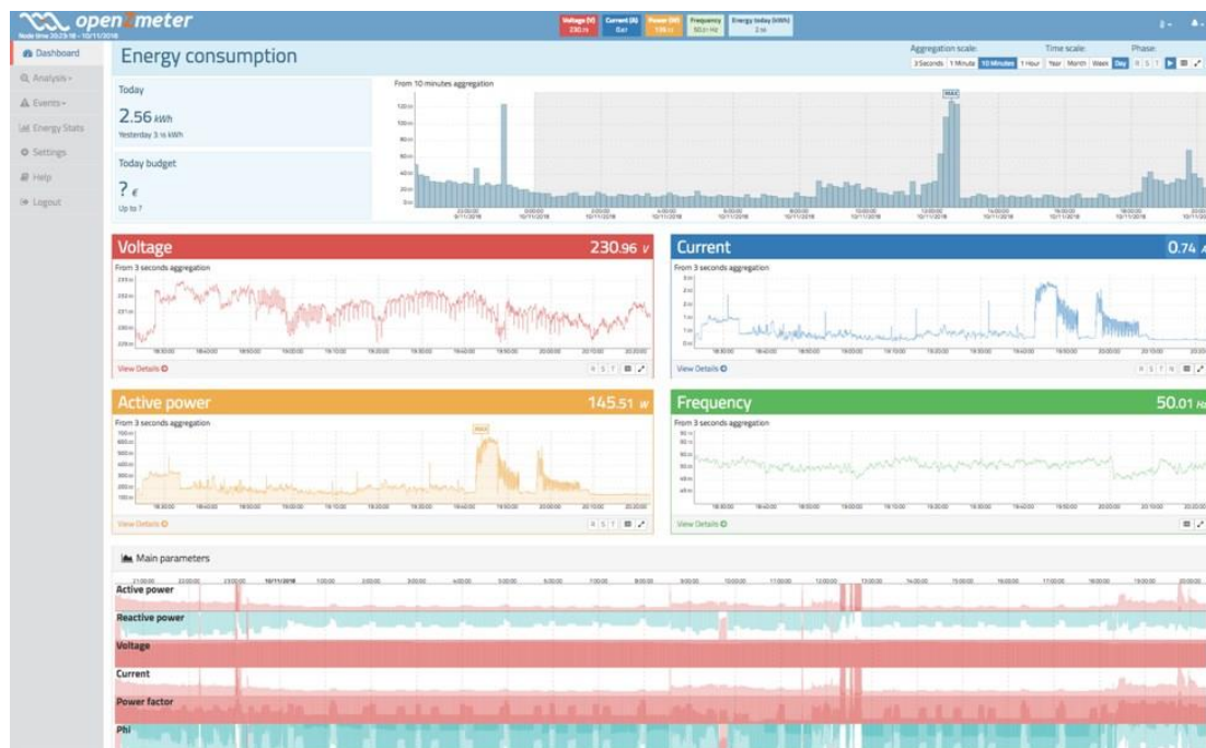
Figure 13 Dashboard of real-time power quality (PQ) monitoring and smart-metering software.
