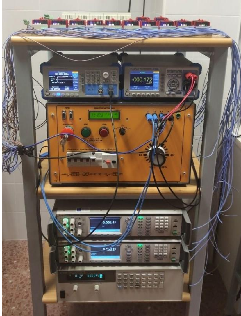
Figure 35 Equipment used to calibrate 3Ph-oZm: On top, some 3Ph-oZm's prepared to be calibrated. A variable three-phase power supply in the middle (Yellow box). Finally, two 8.5 digit high accuracy multimeters Fluke 8558A and an Agilent 6812 digital power supply at the bottom.
