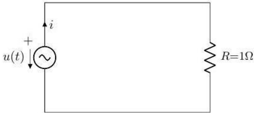
Figure 44 Resistor load and non-sinusoidal source
