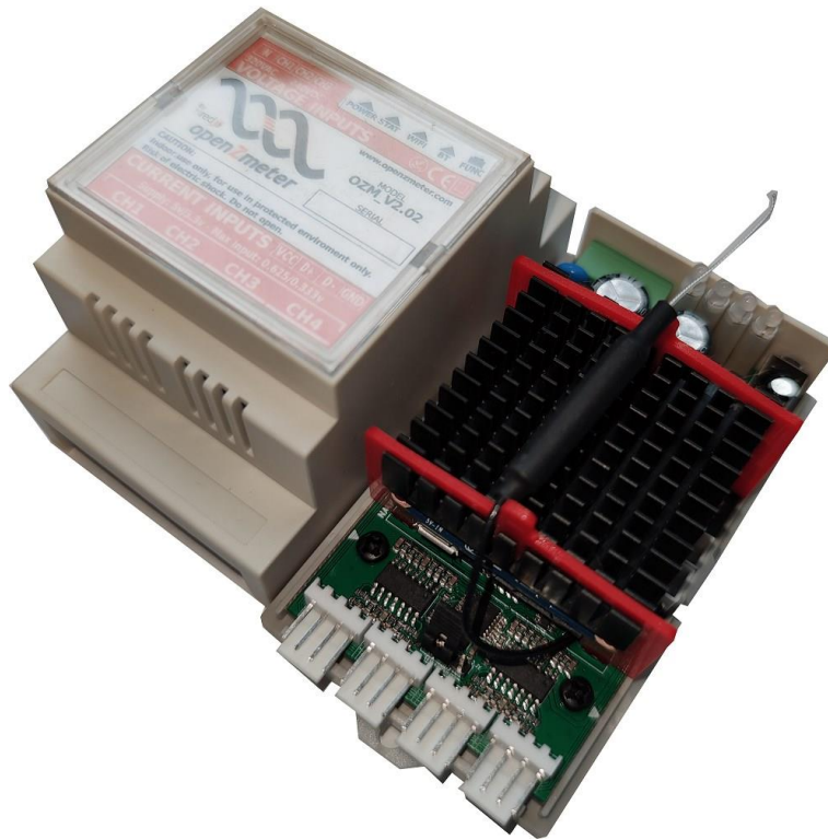
Figure 28 Electronic components layout including the Li-Po battery and heat sink. The enclosure covers the device becoming a very compact one.
