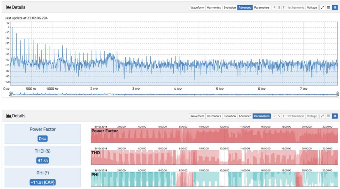
Figure 19 (top) current spectrum. (bottom) advanced parameters THDi, power factor, and phase angle for current.
