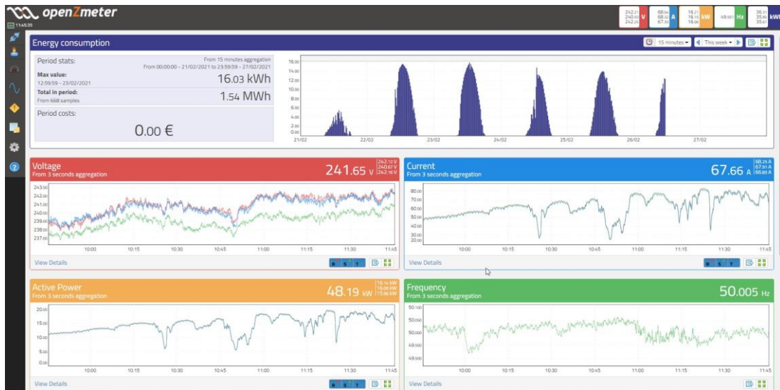
Figure 37 Main dashboard for a real 100kW PV power plant located in Almeria (Spain). This view displays the energy generated and the main RMS values.
