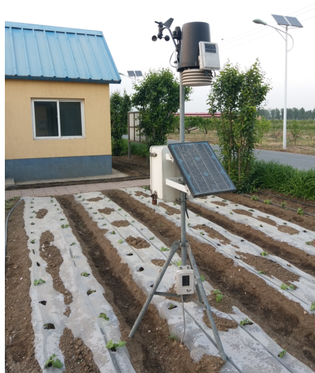
Fig. 1.26. Photo of the outdoor weather station.
