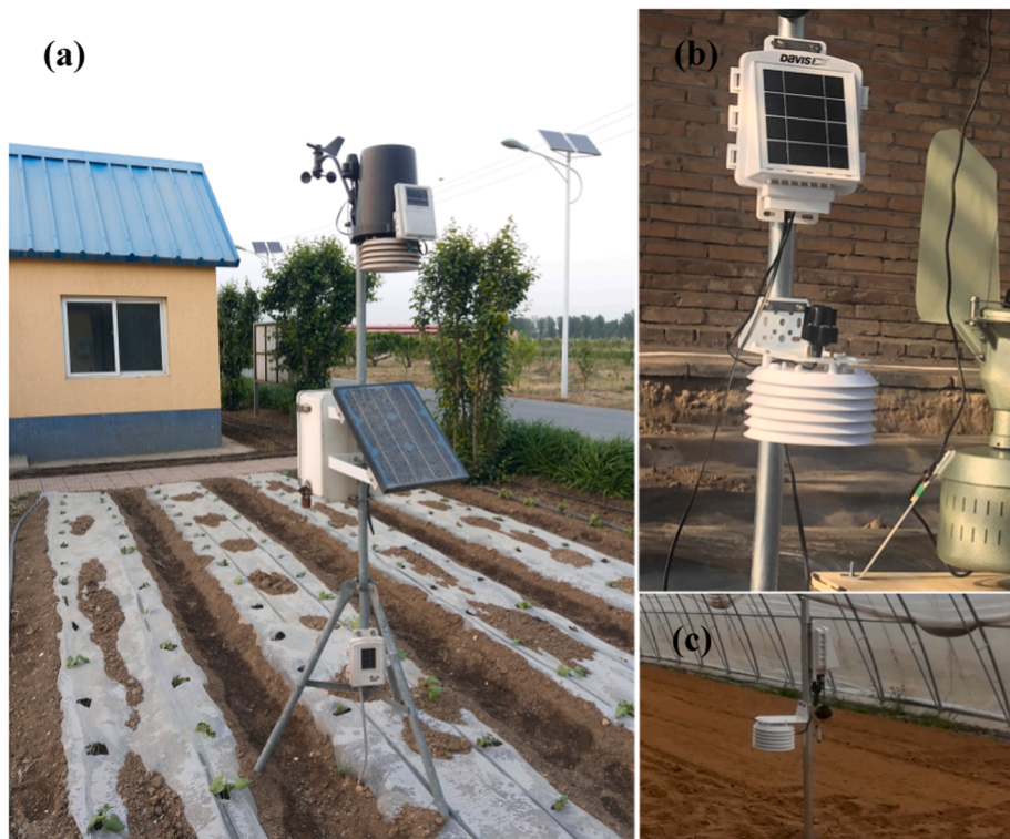
Fig. 3. Sensors used for data collection.
