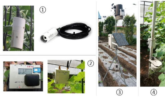
Figure 2. Sensors. (1) SI-111 infrared thermometer; (2) T_a -RH sensors made by NERCITA; (3) Davis Vantage Pro& Plus outdoor weather station; (4) Davis-6162 indoor weather station.
