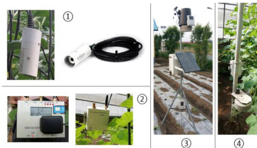
Fig. 2 – Photos of sensors: ① is the SI-111 infrared thermometer; ② is the temperature-relative humidity sensors made by NERCITA; ③ is the Davis Vantage Pro & Plus outdoor weather station; and ④ is the Davis-6162 indoor weather station.
