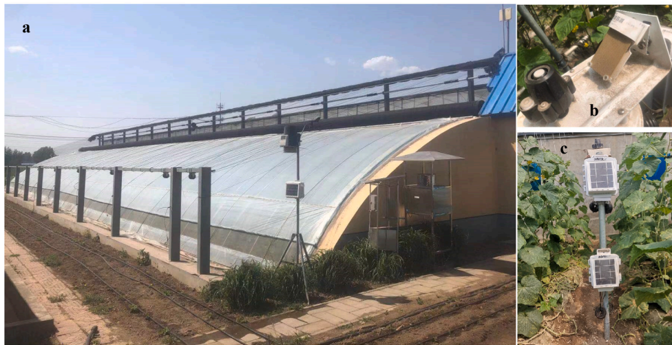
Fig. 1. Experimental greenhouse and outdoor weather station (a); Leaf wetness sensor (b); Indoor weather station (c).
