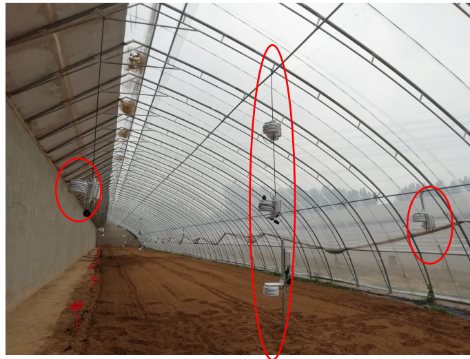
Fig. 1.41. A photo of air temperature and humidity sensors distributed in the greenhouse.
