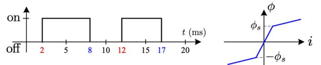
Figure 7. Switching states on/off for circuit in Fig. 6 and nonlinear  $\phi - i$  curve.
