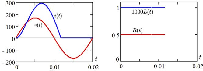
Figure 11. Simulations of a half-wave rectifier. left) Voltage and current; right) Identified  $R$  and  $L$
