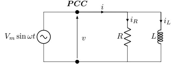
Figure 4. Linear RL parallel circuit with sinusoidal excitation used to illustrate the application of the method.
