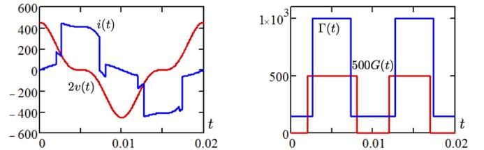
Figure 9. Simulations of nonlinear circuit of Fig. 6 with nonsinusoidal excitation and circuit parameter identification. left) Voltage and current; right) Identified  $\Gamma$  and  $G$ . Compare with Figs. 8(e) and 8(f).
