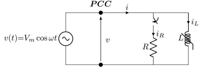
Figure 6. Nonlinear circuit used to illustrate the capabilities of the method to identify circuit parameters
