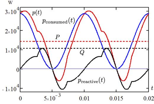
Figure 15. Power quantities for the parallel circuit of Example 2 with linear resistor and saturating inductor.
