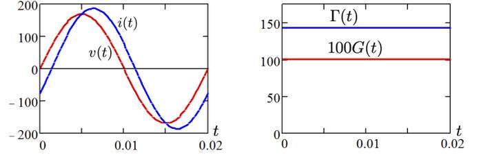
Figure 5. Time variation of parameters for the case of Fig. 4. left) voltage and current vs time at the pcc; right) identified conductance  $G$  and compliance  $\Gamma$ .
