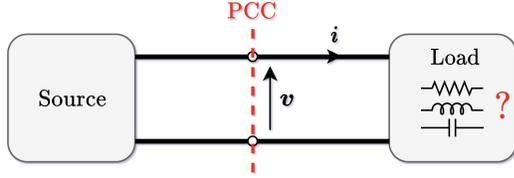
Figure 1. Pictorial representation of the problem solved in this paper.  $v$  and  $i$  are the instantaneous voltage and current measured at the point of common coupling (pcc).
