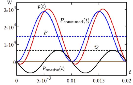
Figure 14. Power quantities for the parallel circuit of Example 1.
