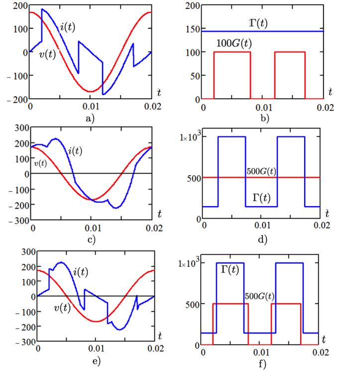
Figure 8. Simulations of nonlinear circuit of Fig. 6 and circuit parameter identification. (a) Voltage and current when the switch operates; (b) Identified  $\Gamma$  and  $G$ ; (c) Voltage and current when the inductor saturates; (d) Identified  $\Gamma$  and  $G$ ; (e) Voltage and current when the switch operates and the inductor saturates; (f) Identified  $\Gamma$  and  $G$ .
