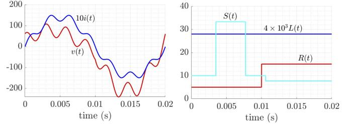
Figure 13. Three parameter identification method with a nonsinusoidal source for a series circuit. left) Voltage and current; right) Identified  $R$ ,  $L$  and  $S$
