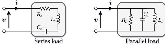
Figure 2. Equivalent circuits for the representation of the load. All variables and parameters are functions of time; left) series equivalent; right) parallel equivalent.
