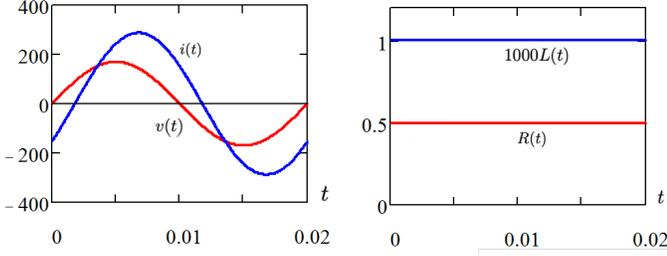
Figure 10. Time variation of parameters for the series RL case. left) voltage and current vs time at the pcc; right) identified resistance  $R$  and inductance  $L$ .
