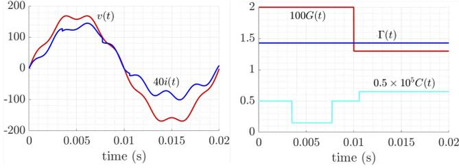
Figure 12. Three parameter identification method with a nonsinusoidal source. left) Voltage and current; right) Identified  $G$ ,  $\Gamma$  and  $C$ .
