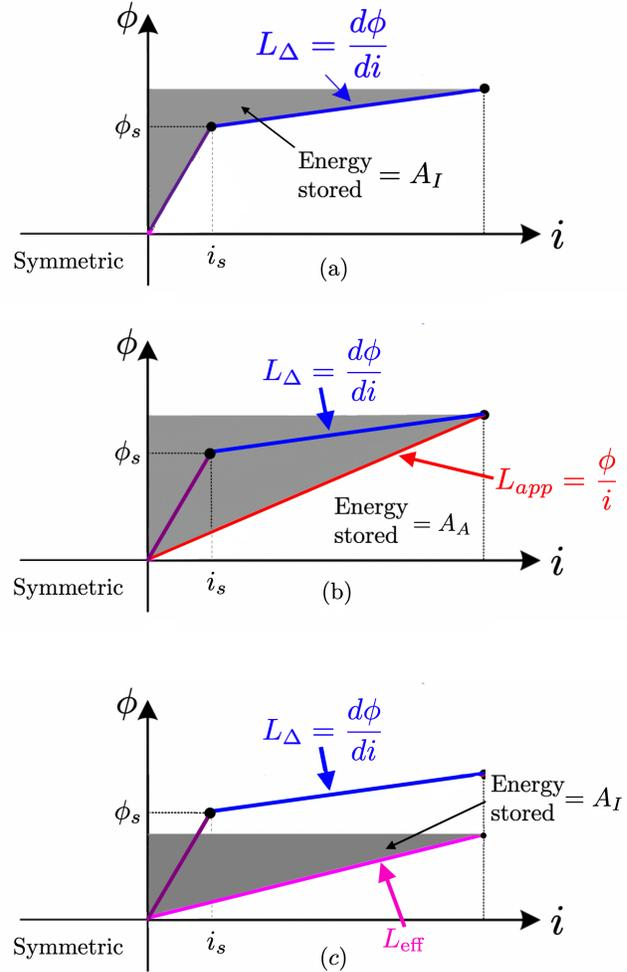
Figure 3. Illustration of the apparent, incremental, and effective inductances for a linear piece-wise variation. In the linear region  $-\phi_s \leq \phi \leq \phi_s$  all inductances are the same.
