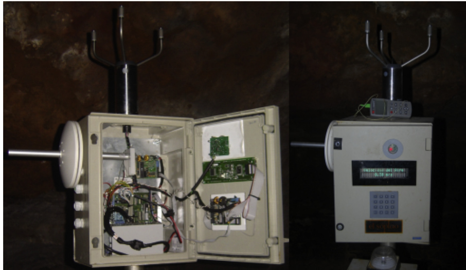
Fig. 10. Inside and outside view of the remote Viento station.
