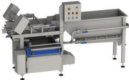
The washed product is transported to the download section where water sprinklers are installed in the final section of discharge giving an additional shower wash to it, which helps to reduce or eliminate chlorine or other additives residues. This final shower can be considered as the wash step which we called rinse in previous sections. Next it is displaced through a small conveyor belt where takes place a small intake of excess of water.
