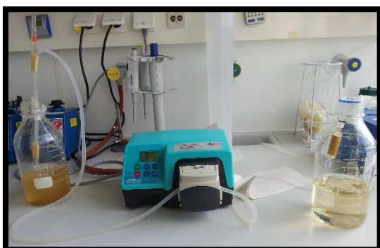
Image 1: Watson-Marlow 323 pump, DNA extraction
