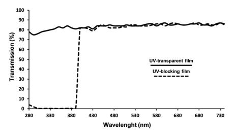
**Figure 1.** Spectral transmission of the UV-transparent and UV-blocking polyethylene films used in this study.
