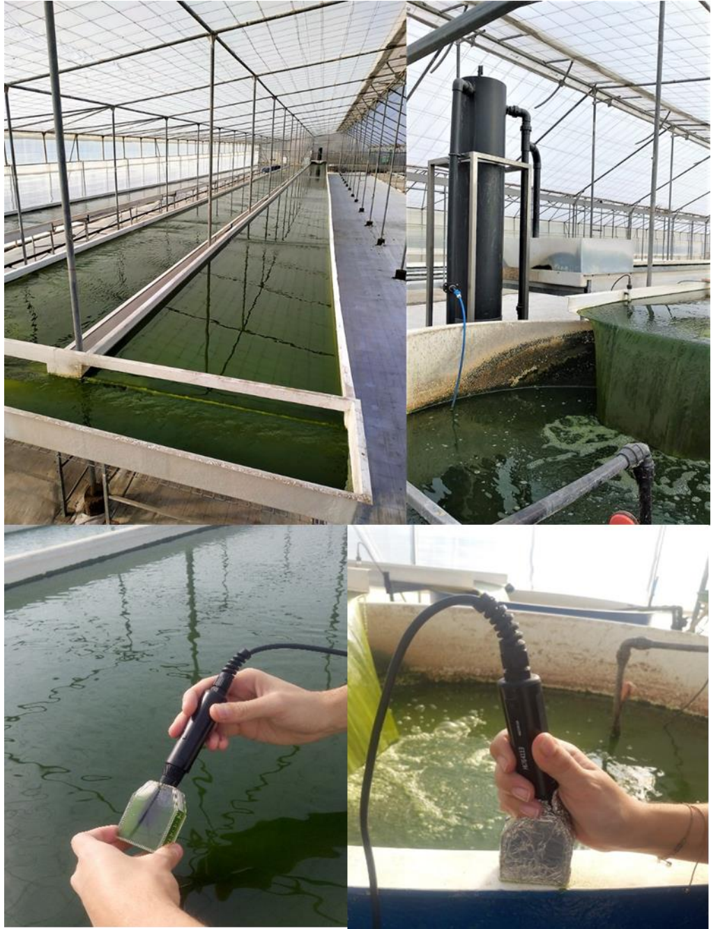
Figure 1.- Images of the thin-layer reactor located at the IFAPA Research Center (Almería, Spain) (Up) and the plastic chamber used to determine the oxygen production and consumption at the different positions (Below).
