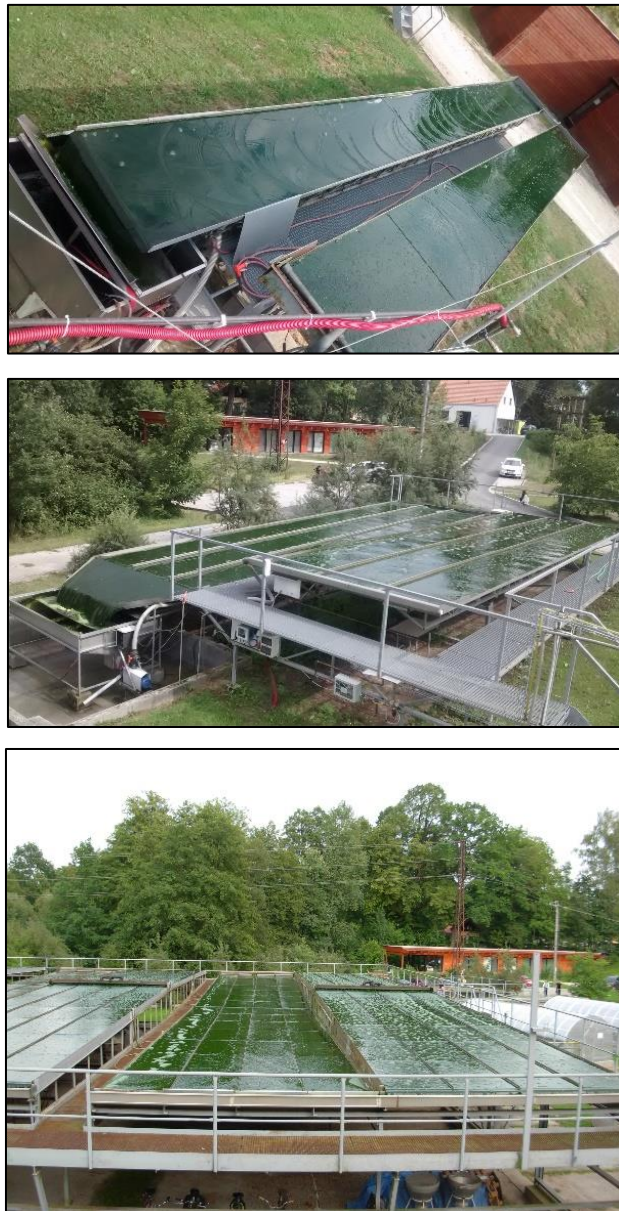
Figure 3.7. General view of the thin layer reactors (A=200 L, B=600 L, C=2200 L) located at the "Algatech" Experimental Station in Trebon (Czech Republic). Pictures from August 2018.
