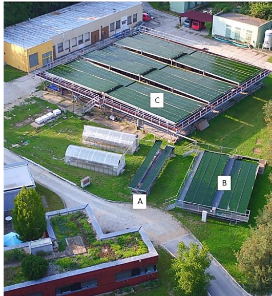
Figure 1. Areal view of the thin layer cascades (small A= 200 L/24 m 2 ; medium B = 600 L/90 m 2 ; large C – three units, each 2200 L/224 m 2 ) located at Centre Algatech in Třeboň (Czech Republic) (detailed description in Masojídek et al. 2011, 2015, Grivalský et al. 2019)
