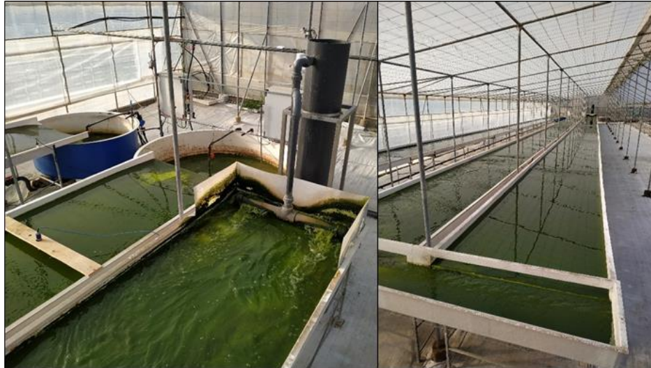
Figure 3.5. General view of the thin layer reactor located at the "IFAPA" experimental station in Almería (Spain) working in continuous mode since June 2018.
