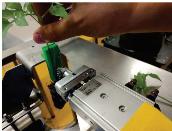
Figure 2. Cutting device. As can be seen, a fitting device is used to guarantee or ensure the verticality of seedling in the cutting process, beside a groove for insertion of the cutting blade. A specific fitting device for each cutting angle was developed. Once inserted, the seedling is dissectioned in two by a sharp blow of the sharp blade.
