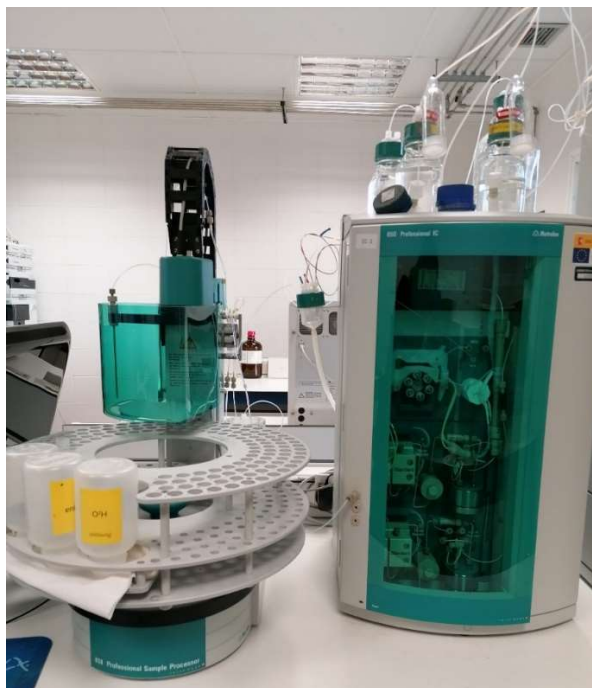
Figure 27. Metrohm 850 Professional IC used for the determination of ionic species contained in water samples.
