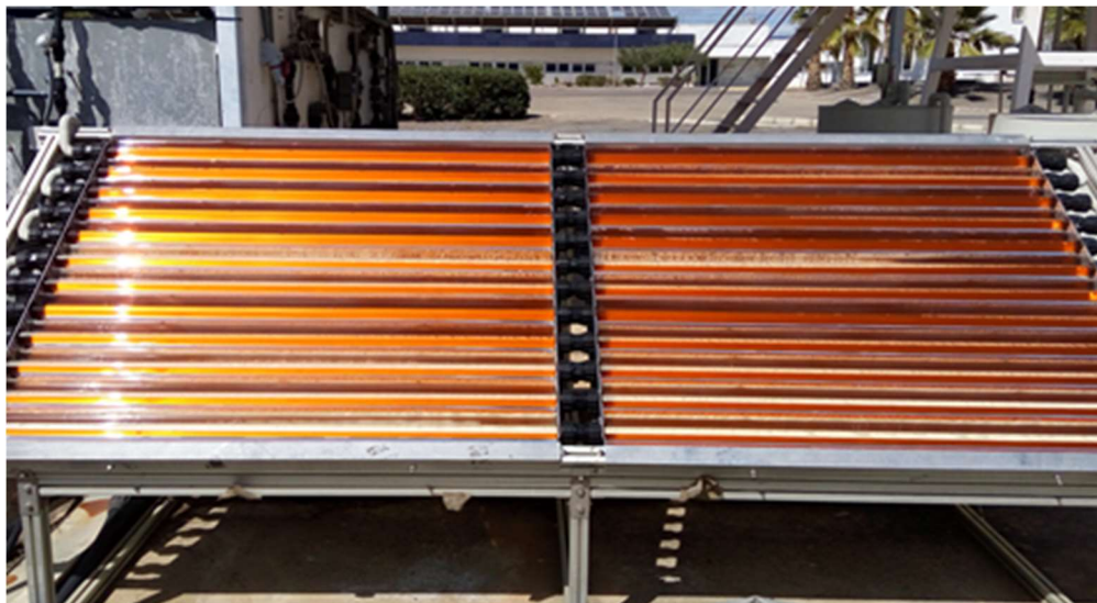
Figure 38. Solar CPC photoreactor combined with the electrochemical device during the treatment of a landfill leachate in the facilities of PSA.
