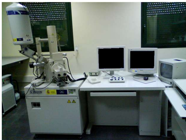
Figure 28. Hitachi S-3500N SEM and Oxford INCAx-sight EDX at University of Almería.
