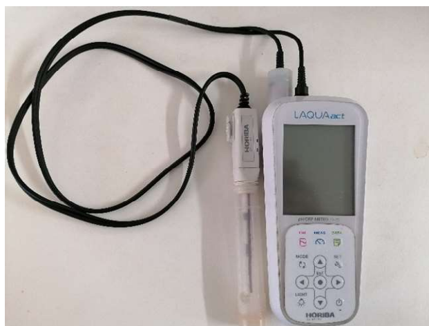
Figure 14. Portable pH-meter LAQUAact PH110 used for pH determinations.
