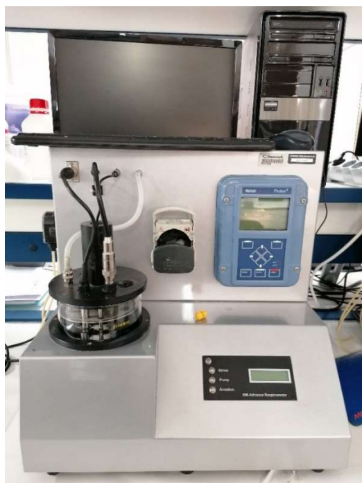
Figure 24. SURCIS BM-Advanced Respirometer used to perform toxicity and biodegradability assays
