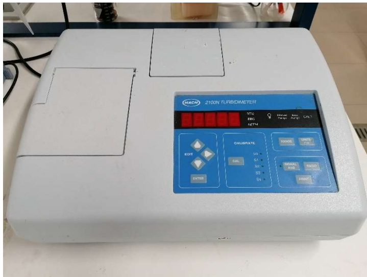
Figure 16. Equipment for turbidity measurements (2100N turbidimeter from Hach) available in the Water Technologies Laboratory at PSA
