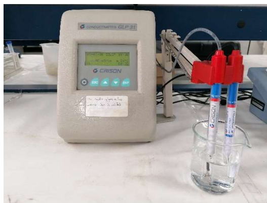
Figure 15. Conductivity meter available in the Water Technologies Laboratory at PSA.
