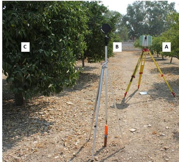
**Figura 5. 9. High definition survey (HDS) in the trial. (A) HDS Station. (B) Ranging rod and tripods placed on the stakes. (C) Orange Trees**
