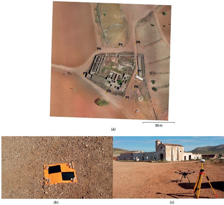
Figure 9. GCPs used for the georeferencing of the photogrammetric project: (a) distribution of GCPs; (b) example of target; (c) GNSS used in this work.
