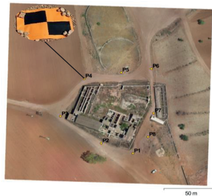
Fig. 4. Distribution of GCPs for the georeferencing of the photogrammetric project, overlapped to orthoimage obtained from photogrammetric project Two flights were made; the first at a height of 50 m above ground level, with an autopilot using the DJI GS Pro © application to obtain nadiral photographs. The flight plan consisted of 11
