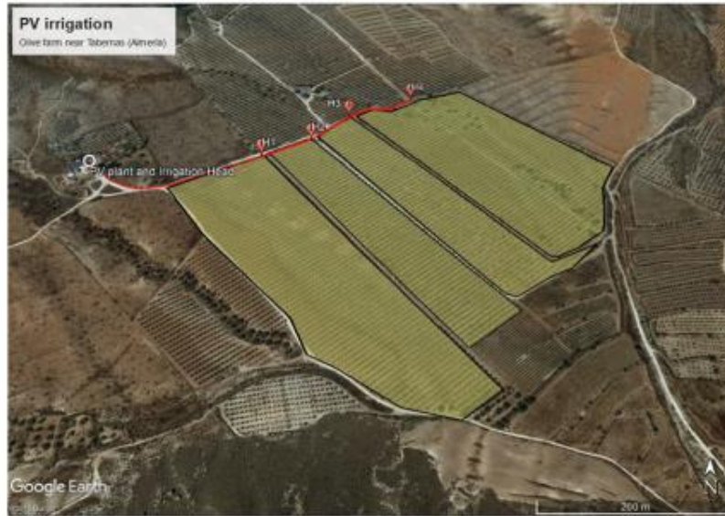
Fig. 4. Layout of the experimental farm and PV irrigation system.
