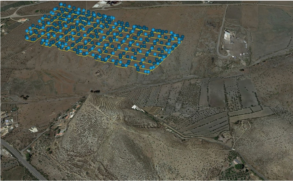
Figure 6. Example of the route followed by the drone for the 50-m height flight.
