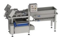
The washed product is transported to the download section where water sprinklers are installed in the final section of discharge giving an additional shower wash to it, which helps to reduce or eliminate chlorine or other additives residues. This final shower can be considered as
