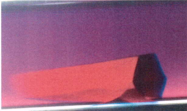
Fig. 5 – Photograph of a B-PE crystal grown via the capillary counter-diffusion technique from a purified fraction obtained in the VFR.
