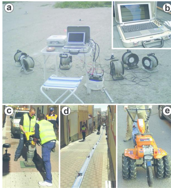
Fig. 2. (a) SPAC sensors deployment at an open site. (b) SPC-35 digitizer. (c) Portable vibrator seismic source. (d) Land-streamer system with the geophones being towed through streets. (e) Small tractor situated at the head of the land-streamer to easily move all the system.
