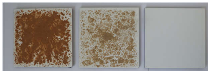
Figure 5. Picture of the set of samples after the sand deposition, with sand from Ouarzazate (left), with sand from Dubai (center), and without sand (right).
