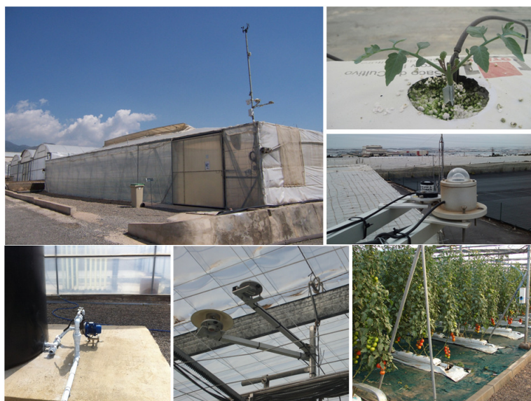
Figure 3. Greenhouse facilities used for the experiments performed in this work. From left to right and from top to bottom: greenhouse, dropper, solar and PAR radiation device at the outside, irrigation system, solar and PAR radiation device inside the greenhouse and the tomato crop lines.
