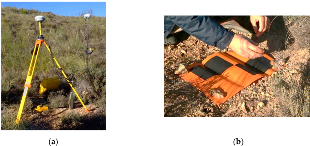
Figure 5. Surveying campaign: (a) Trimble R6 Rover and base GNSS receivers; (b) target for the ground control points (GCPs).
