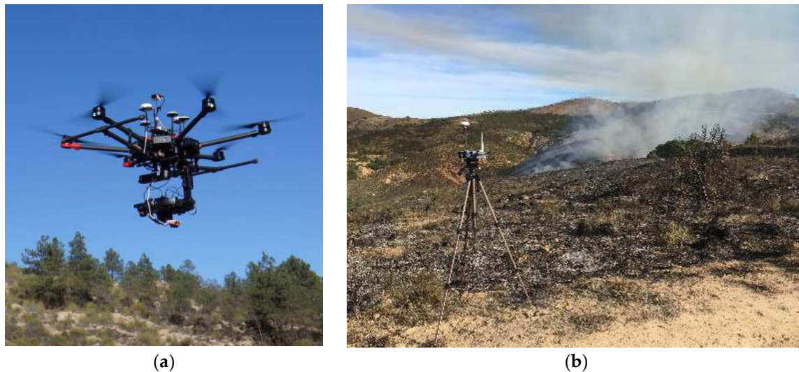
Figure 3. Unmanned Aerial Vehicle (UAV) system: (a) DJI Matrice 600 Pro with a Parrot Sequoia multispectral camera onboard and D-RTK navigation antenna; (b) Base station of the D-RTK Global Navigation Satellite System (GNSS) positioning and navigation device.
