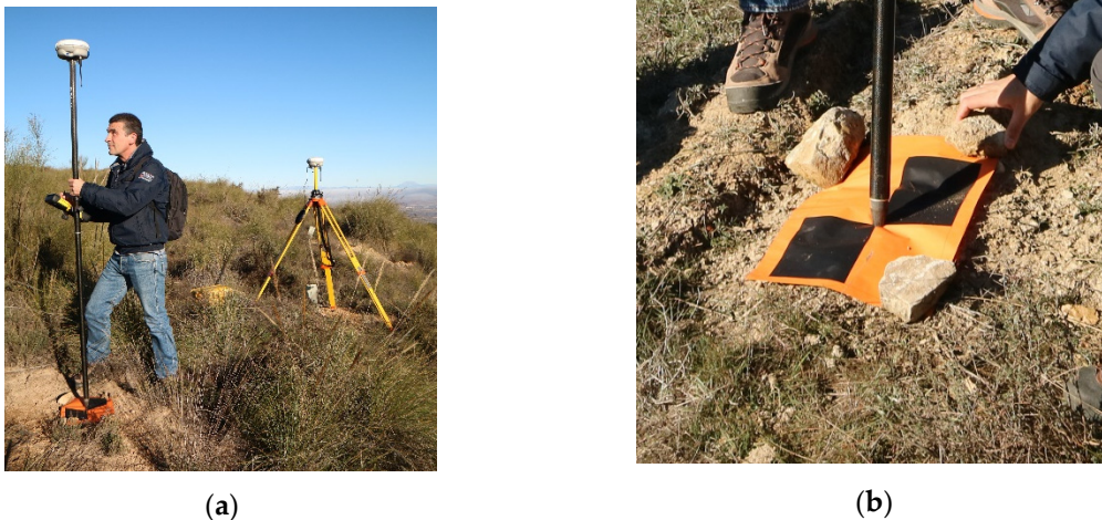
Figure 6. Surveying campaign: (a) Trimble R6 Rover and base GNSS receivers; (b) target for materializing the ground control points (GCPs).
