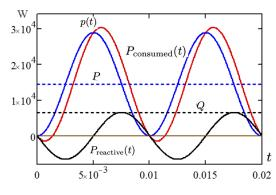
Figure 14. Power quantities for the parallel circuit of Example 1.
