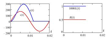
Figure 11. Simulations of a half-wave rectifier. left) Voltage and current; right) Identified R and L
