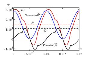
Figure 15. Power quantities for the parallel circuit of Example 2 with linear resistor and saturating inductor.
