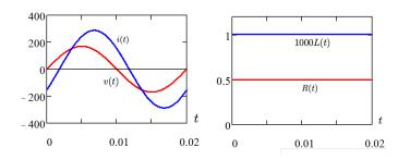
Figure 10. Time variation of parameters for the series RL case. left) voltage and current vs time at the pcc; right) identified resistance R and inductance L.
