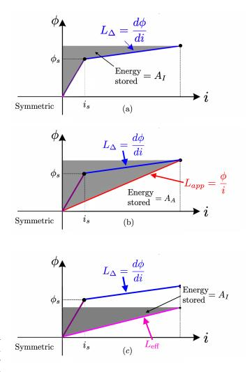
Figure 3. Illustration of the apparent, incremental, and effective inductances for a linear piece-wise variation. In the linear region  $-\phi_s \leq \phi \leq \phi_s$  all inductances are the same.
