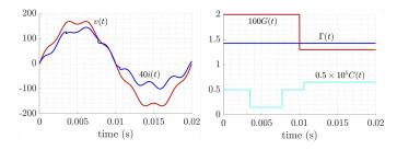
Figure 12. Three parameter identification method with a nonsinusoidal source. left) Voltage and current; right) Identified G,  $\Gamma$  and C.
