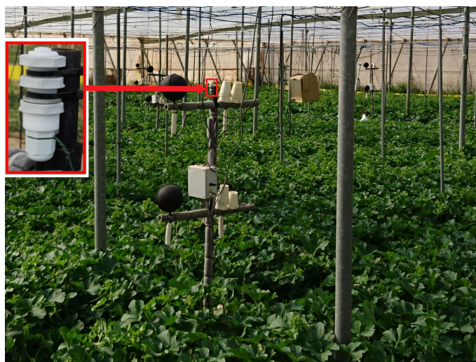
Figure 2. Interior of the greenhouse studied and detail of one of the sensors installed for the measurement of UV radiation.
