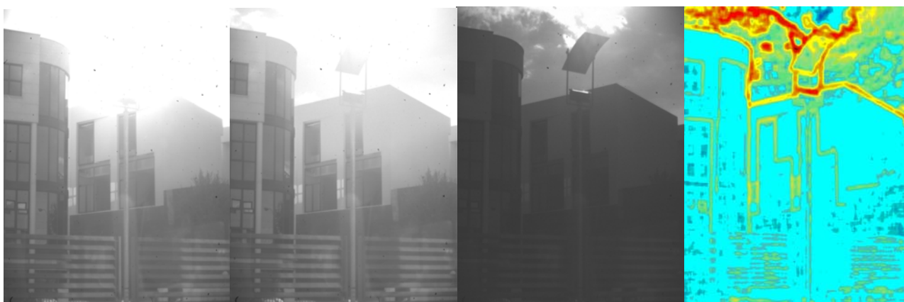
Figure 8. Different images taken from a scene with increasing values of V_1 and V_2 from left to right. The last image on the right shows the local entropy map of the image on its left (maximum values in red, minimum values in blue).
