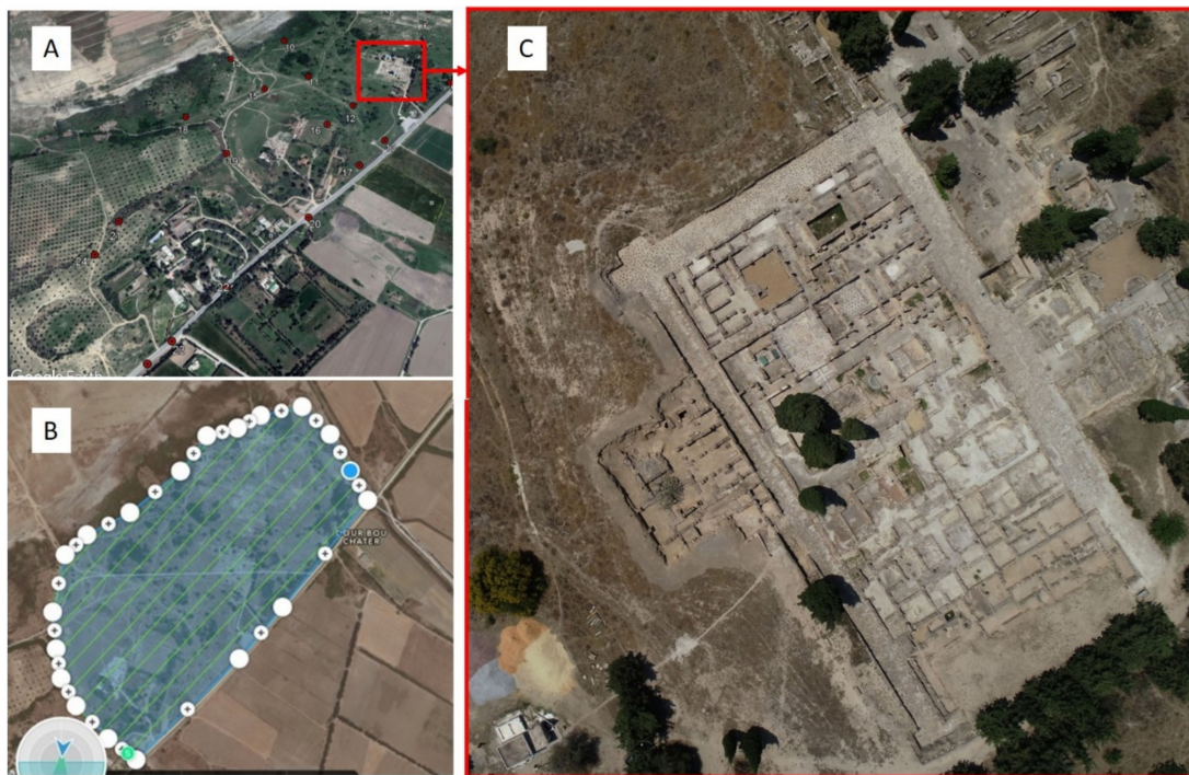
Figure 15. UAV photogrammetric flight of Utica (Tunisia). (A) Ground control points. (B) Photogrammetric flight paths. (C) Example of aerial photography on the restored Roman insula.
