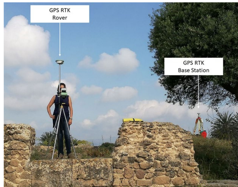
Figure 19. Measurement of control points with GPS RTK for photogrammetric flight in the city of Utica (Tunisia).
