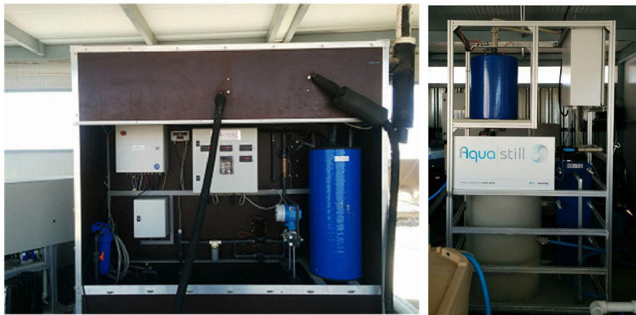
Fig. 7. Commercial MD modules at PSA. From left to right: Solar Spring and Aquastill modules.
