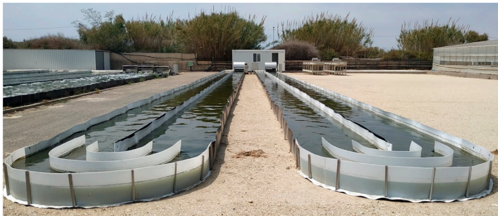
FIGURE 2 | Raceway reactor. The real input data for simulating the seasons of the year were collected from the sensor located in it.
