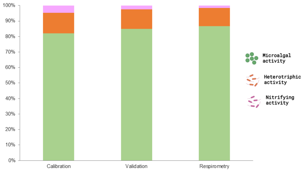
Figure 18.- Microbial percentages obtained during the calibration process, validation process and experimental photo-respirometric trials.
