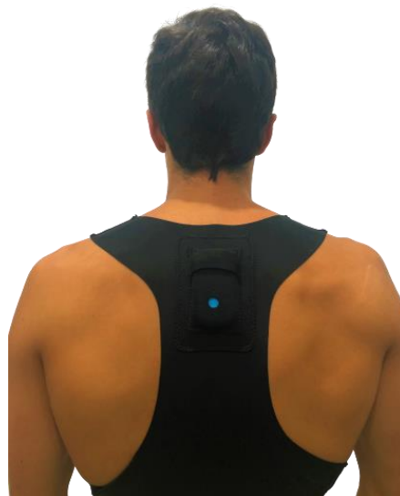
Figure 24. Tracking system placed in the back pocket of a chest vest
