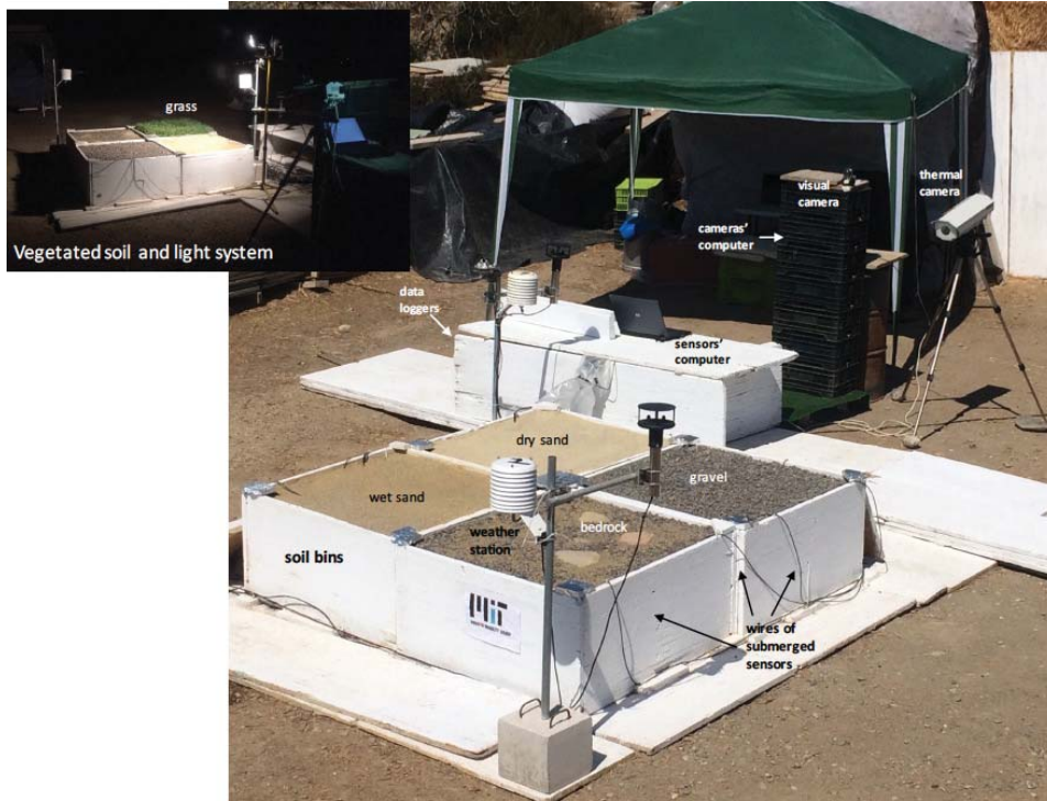
Figure 1: Testing site specifically built for these experiments. Notice the modular and scalable configuration of the soil bins as well as the accessible disposition of the place for setting sensors and hardware. Observe, at the top left corner, the second configuration of this testing site with a soil bin with grass (top right corner) and the artificial lighting system used at night
