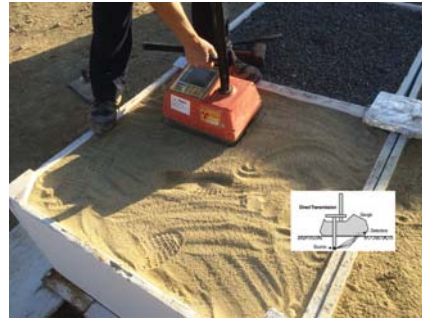
(c) Bedrock. USCS: Well-graded sand (SW) (d) Nuclear density meter
