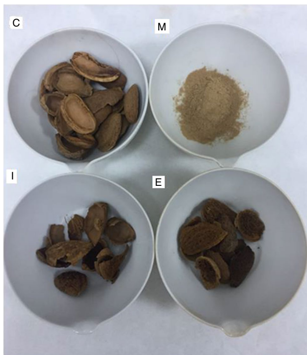
Fig. 3 Several selected sample materials of almond shells placed in the ceramic crucibles prepared by thermal treatments in air: Sample C, Sample M, Sample I and Sample E
