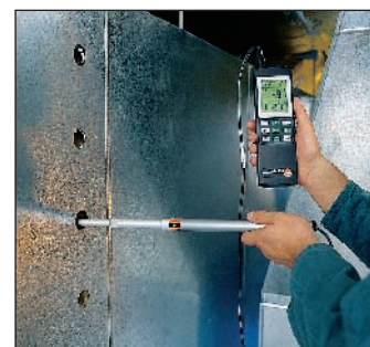
Volume flow measurement using timed and multi-point mean calculation
