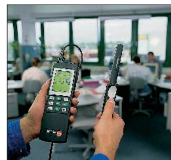
Monitors indoor air quality with CO2 probe
