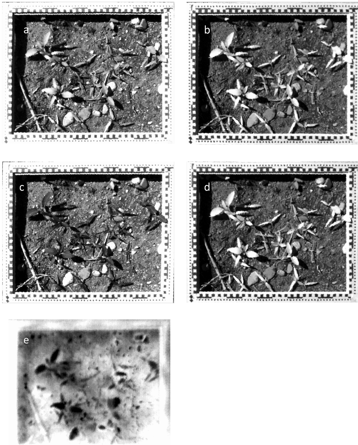
Fig. 12. Rectified bands of sample 9: GRE (a), NIR (b), RED (c), REG (d), THE (e).
