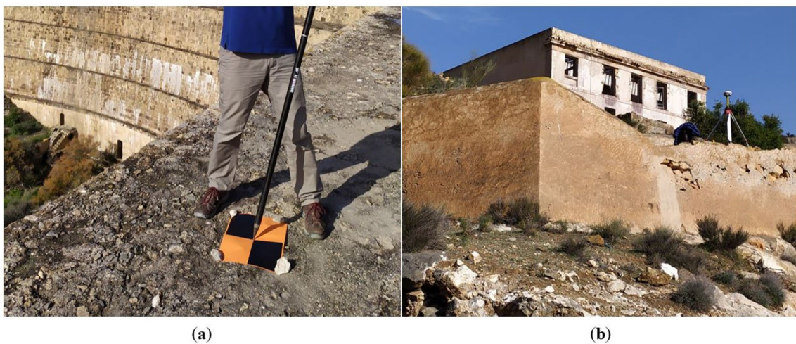
Fig. 6 a One of the targets used in this work; b GNSS receiver base applied to this work
