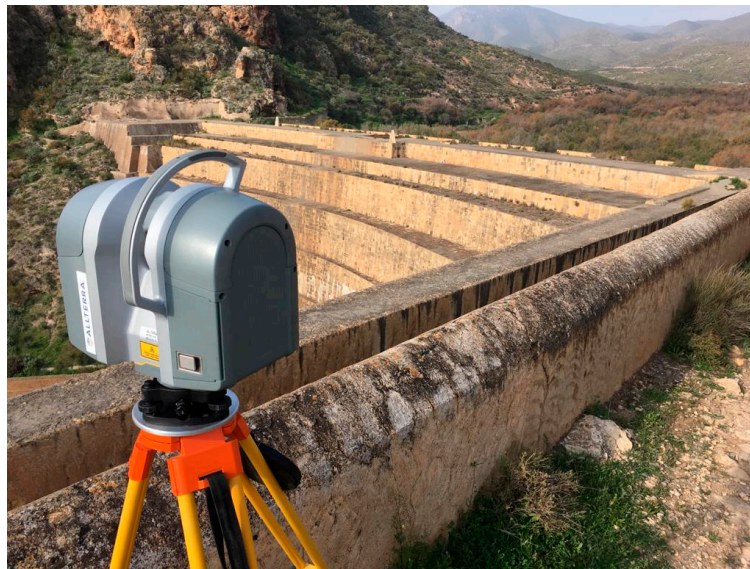
Figure 6. Trimble TX-8 Scanner.
