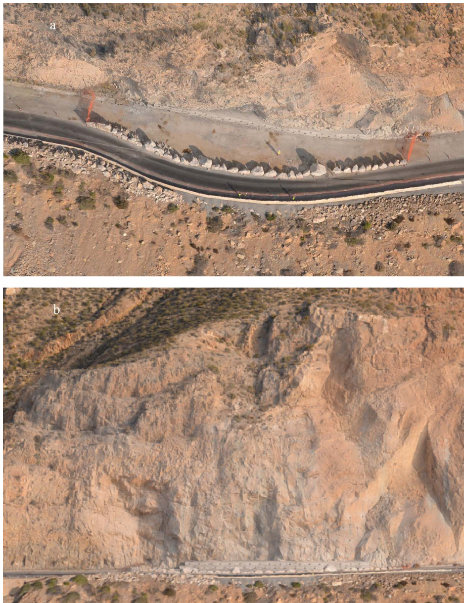
Fig. 10. Orthophotos obtained using a horizontal projection plane (a), and using the plane that has been fit to the point cloud generated during the photogrammetric process (b).
