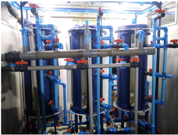
Fig. 2 Photograph of the pilot-scale algal–bacterial biofilter
