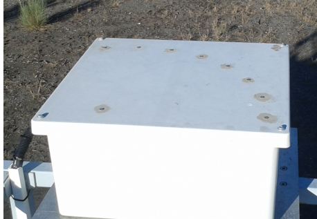
Figure 5: CSS at PSA. The 9 dots, 8 arranged in a circular arc around one in its center, are the sensors used to determine cloud shadow speeds and directions.
