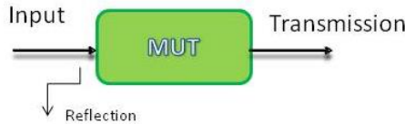
Fig. 3 - Transmission and Reflection of the Material Under Test.
