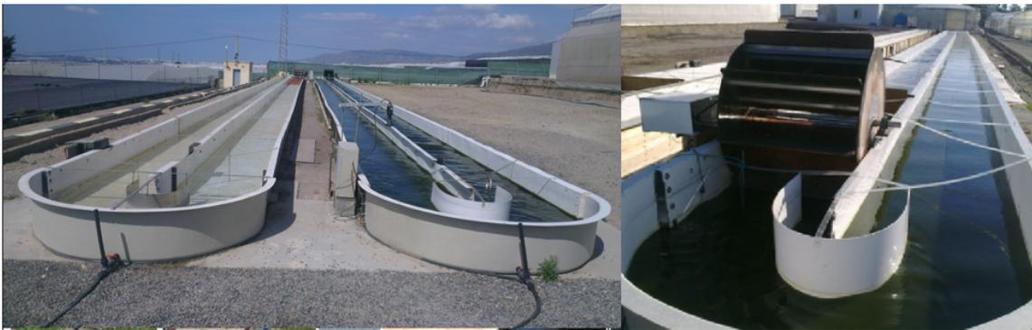
**Figura 2.2:** Fotobiorreactor industrial raceway
