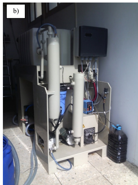
Fig. 2. Aquaver's MDS-40B prototype: a) lateral view, showing the auxiliary distillate tank, and b) front view, showing the brine and distillate vessels of the unit and the control panel.
