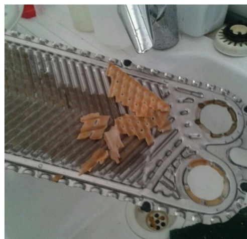
Fig. 14. Slabs of scaling over a plate of the heat exchanger of the desalination unit.
