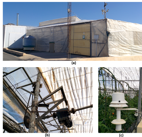
Figure 1. Experimental greenhouse: (a) Exterior view in which roof and side vents can be observed. (b) Motor for the roof vents. (c) Inside air temperature and humidity sensor protected with a solar radiation shield.
