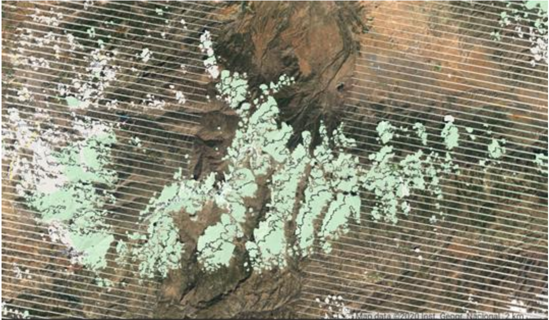
Figure 3.3. Effect of Scan Line Corrector fault on Landsat7 imagery in Sierra Nevada (Spain) and data gaps due to clouds (in green and white). Landsat-7 image courtesy of the U.S. Geological Survey.
