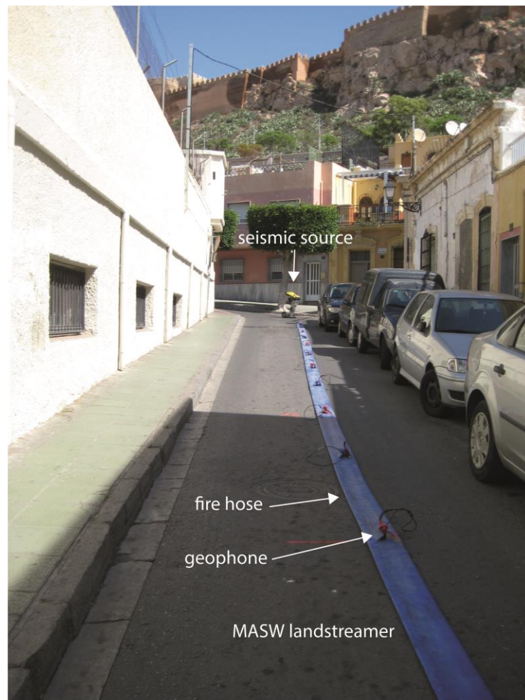
Figure 4. MASW landstreamer layout through Almeria city streets, with the seismic source at the back of the acquisition system.
