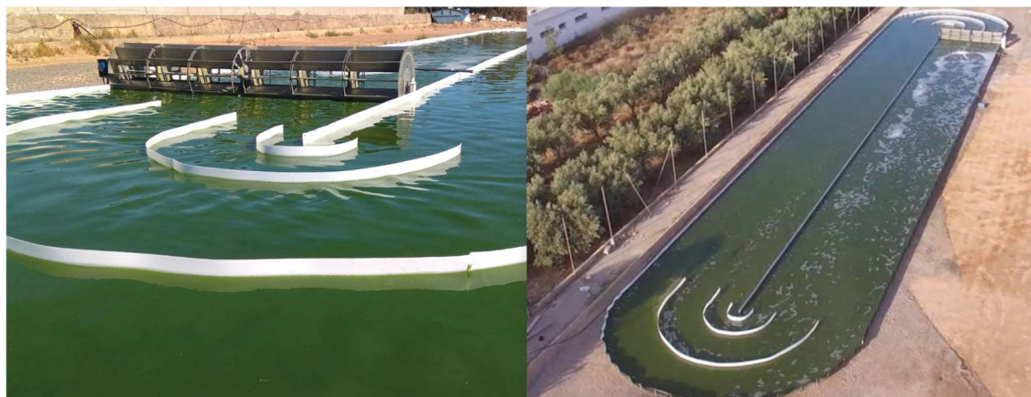
Fig. 1. Images of the real raceway reactor utilized, it being already installed at Las Palmerillas Experimental Station, Almería. Spain.
